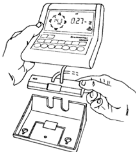
Placing Data Logger Inside Base
